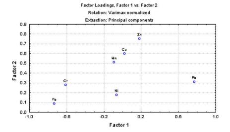
Fig. 2 Principal component analysis applied to metals content in soil samples loading values of the initial variablesy
